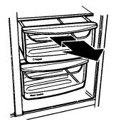
Pull out to the stop, lift the front, and pull again.
